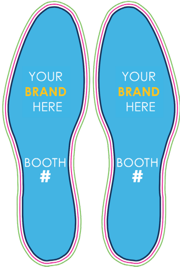
Green line - background art with bleed Blue line - Live art limits (text, logos, etc) Pink line - Trim line
